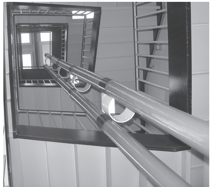
Fig. 2 A 7 m multi-beam inflated free standing structure designed and installed in a stairwell.
