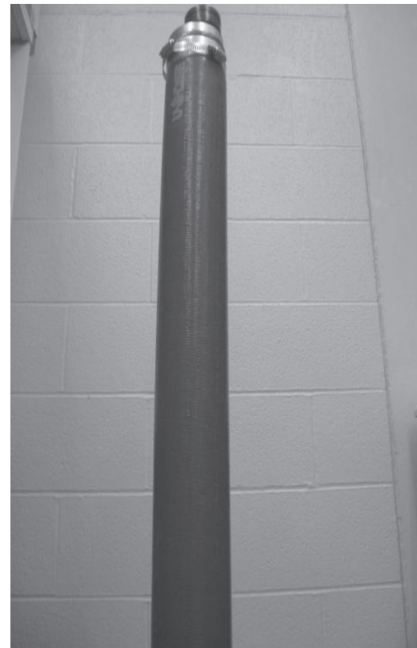
Fig. 3 (a) Inflatable non-tapered tower divided into a number of sections having the same pressure and (b) Free standing beam inflated by an air compressor.
